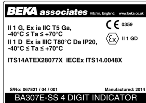
BA307E-SS intrinsic safety certification label
