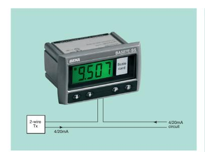
The BA507E-SS rugged general purpose. panel mounting 4/20mA loop powered Indicator, has a stainless steel housing allowing it to be safely installed in harsh industrial and marine environments, or where the front of the instrument is likely to be impacted. Incorporating a full 4 digit display with guaranteed performance between -40 and 70°C, the indicator can be calibrated to show the 4/20mA input current in almost any engineering units.
