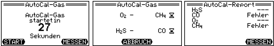
AutoCal adjustment with test gas mixture not successful (e.g. due to wrong test gas concentration)
