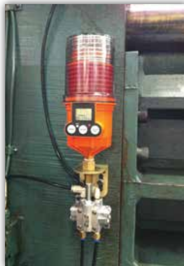
Streamliner M unit with a 4-outlet distribution block
