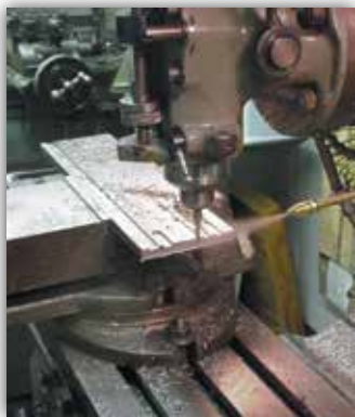
Spray cooling during milling operation
