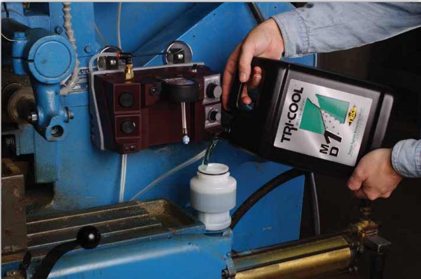
Micro-dispenser being filled with Tri-Cool MD-1 lubricant
