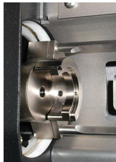
Large Vial Insert Installed
