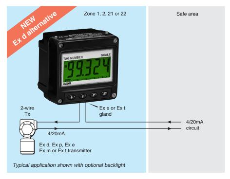
The BA324SG loop powered 4/20mA indicator is a new low cost alternative to a flameproof Ex d indicator featuring a large 29mm high display. Increased safety Ex eb and dust ignition protection by enclosure Ex to certification allow it to be safely installed in Zones 1, 2, 21 or 22 without the need for a Zener barrier or a galvanic isolator. Installation requirements are the same as those for an Ex d instrument.
