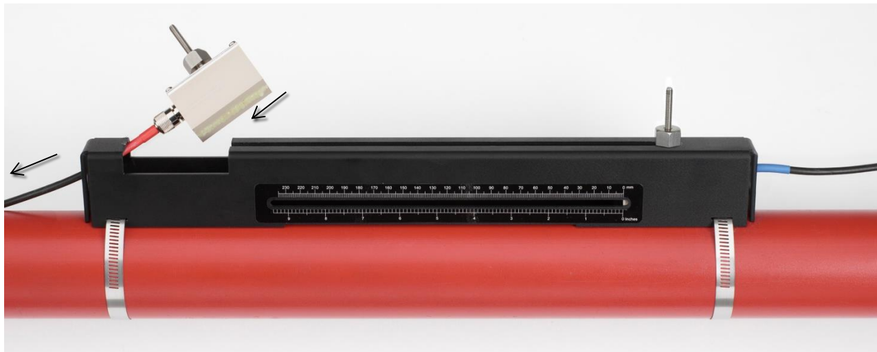
Figure 15 Installing upstream transducer (red)
