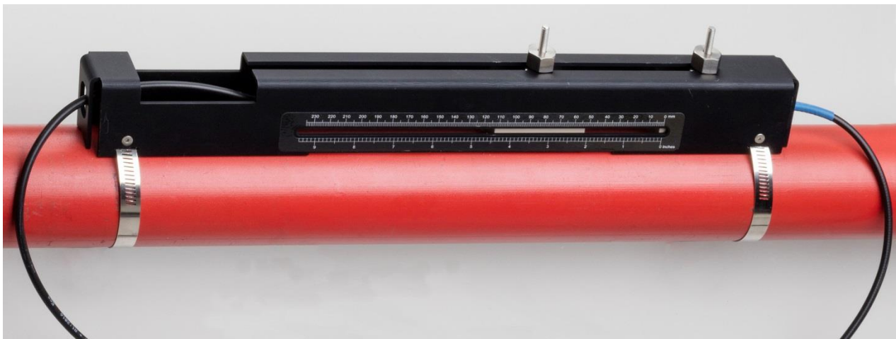
Figure 17 Lowering transducers onto pipe
