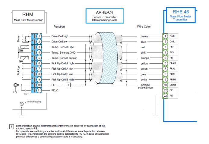
Make sure that you connect the associated RHM to the RHE. See type plate of the RHE for the serial number of the associated RHM at "Set for".
