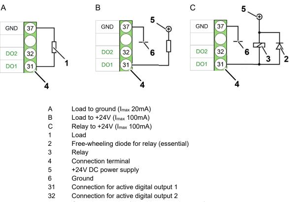
37 Ground connection (digital inputs and outputs)
