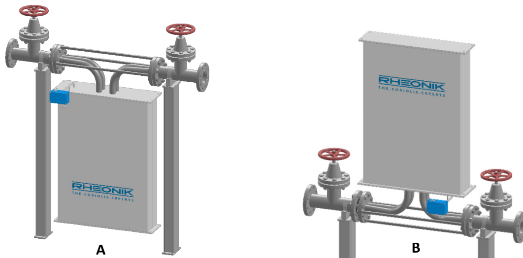
Figure 8: Installation positions for liquid (A) and liquid applications with solid particles/gas applications (B)
