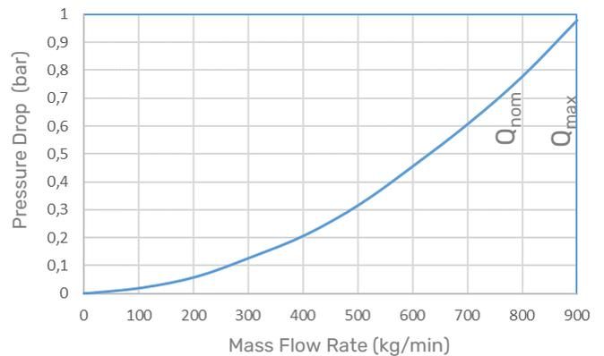
0 – 900 kg/min water, sensor with P1 pressure rating. Higher viscosities create higher pressure drop
