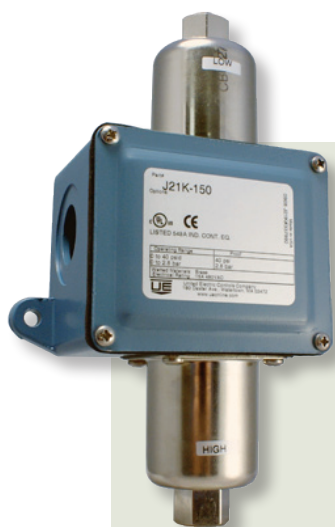
J21K-254 differential pressure switch with brass pressure connections and phosphor bronze bellows
