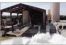
Our large volume test facility is located in Porterville, California. This facility is one of the world's largest volumetric test facilities owned by a meter manufacturer, and it offers accuracy and calibration tests of flow meters from 3 to 72-inch diameter, with flow rates up to 60,000 gpm.
