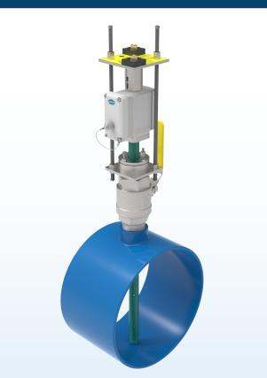
The FPI Mag operates based on Faraday's Law of Electromagnetic Induction: When water (a conductor) moves through a magnetic field, it produces a voltage that is directly proportional to the velocity of the conductor.
