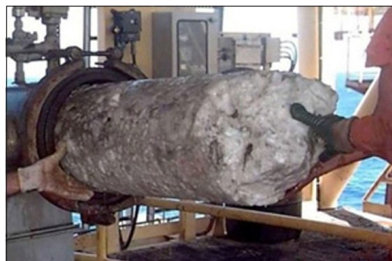
Gas hydrate blockages formed in a subsea hydrocarbon pipeline..
