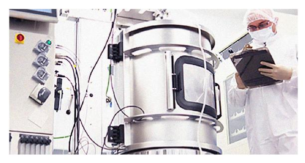
The pharmaceutical industry uses fermentation process in Bioreactor vessels to grow microorganisms that are used in antibiotics, vaccines, steroids, etc...
