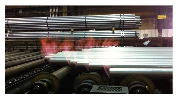
Heat treatment processes for metals represent harsh environments for the measurement of blanket gas constituents. Ambient conditions in the furnaces have high particulate levels, acid gases and other compounds either outgassing or being burned off of the metal components being processed.
