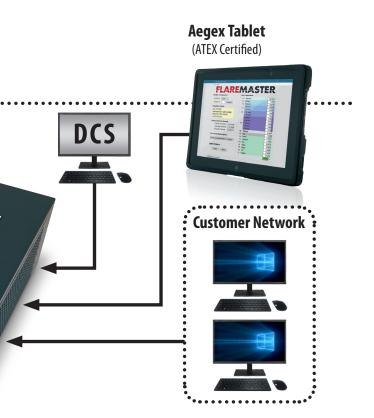
additional redundancy and an advanced software feature set. This imbues the FGM with sustainability of measurement and optimum accuracy under all process conditions, including extreme flare stack blowdown, which can involve flow velocities of up to 1000m/sec. In this configuration, the FlareMaster provides the full dual redundancy, supervisory system referenced above.
