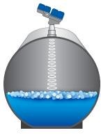
by factoring in tank height and other configuration information. FMCW captures its process variable information in the frequency domain, which supports more accurate signal conversion. The main advantage of FMCW is that it utilises higher receiving sensitivity and higher-strength signals over pulse systems, allowing it to perform better in demanding situations where they may be turbulence, foam or aggressive vapours.
