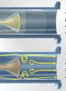
As the flow approaches the cone, the flow profile flattens toward the shape of a well developed profile - even in extreme flow conditions.
